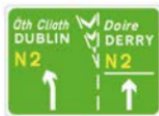
Lane destination sign
