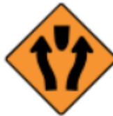
Obstruction between lanes
