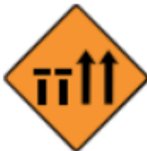
Two nearside lanes (of four) closed
