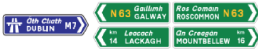
Motorway direction sign
