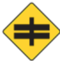
Crossroads with dual carriageway
