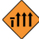
Nearside lane (of four) closed
