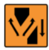
Lanes diverge at crossover
