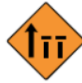
Two offside lanes (of three) closed
