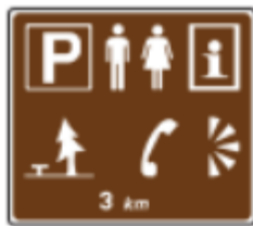
Advance sign for facilities in lay-by
