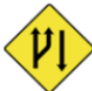
Start of a climbing lane
