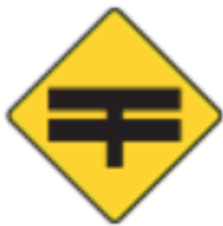
T-junction with dual carriageway
