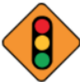
Temporary traffic signals ahead
