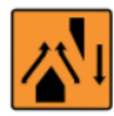
Lanes rejoin at crossover
